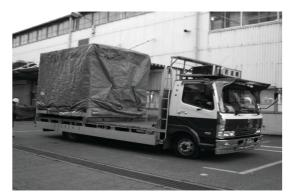
**Figure 12** Transporting a volumetric module of Sekisui House (Source: Hall, Target Magazine, Second Issue 2008, <u>www.ame.org</u>)
