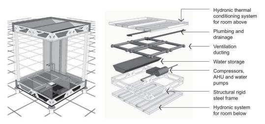
**Figure 2** Volumetric prefabricated material example (Source: Luther, 2009; Multihouse and Digitales Bauen, 2009)
