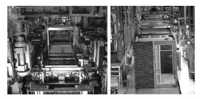
Figure 9 and 10 Volumetric module's production line in Sekisui House (Source: Hall, Target Magazine, Second Issue 2008, <u>www.ame.org</u>)
