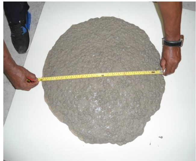
Fig. 8. Slump flow spread.
