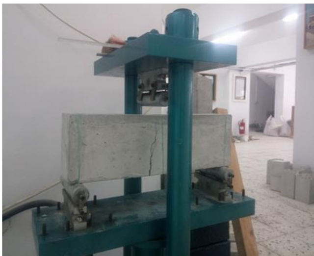
Fig. 5. SFSCC prisms tested for flexural strength.
