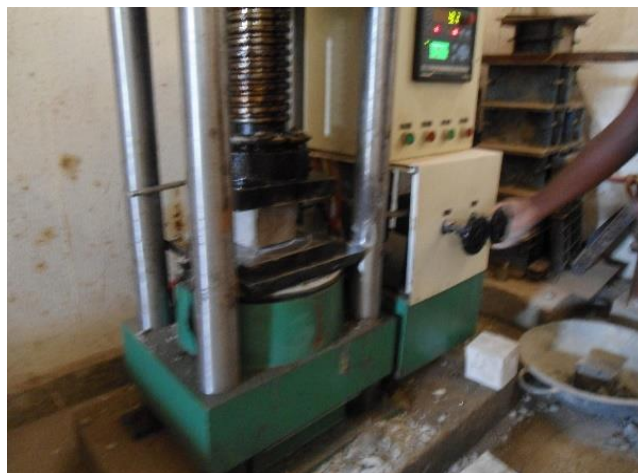
Fig. 3. Compressive strength test.
