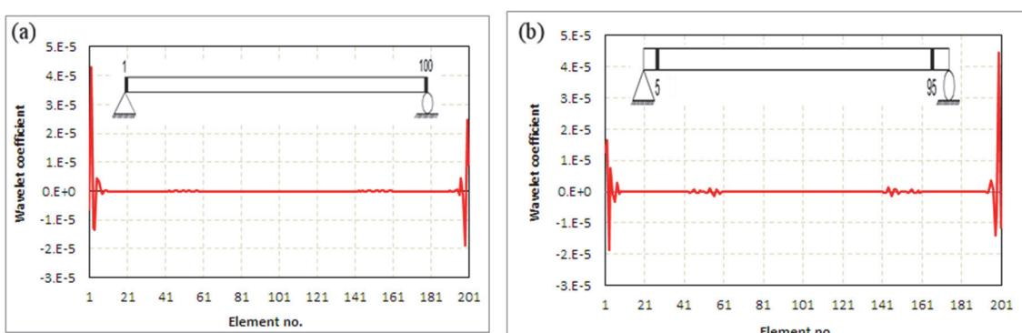
Figure 3: Damage detection using wavelet for scenario no.3. Damages in elements 1 and 100 (a), and Damages in elements 5 and 95 (b).
