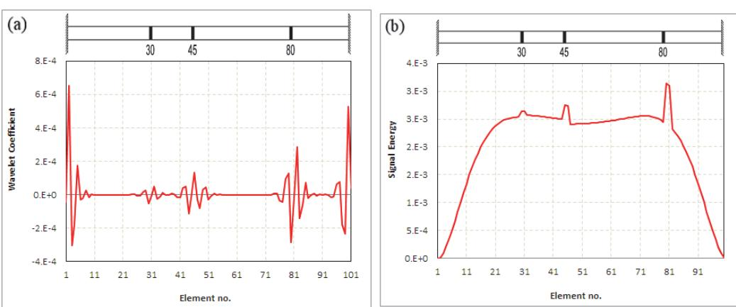
Figure 7: Damage detection using wavelet transform for scenario 9 (a), and signal energy for scenario 9 (b)
