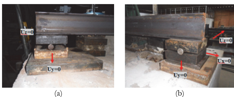
Figure 6: Support conditions of the steel beam specimen [15].
