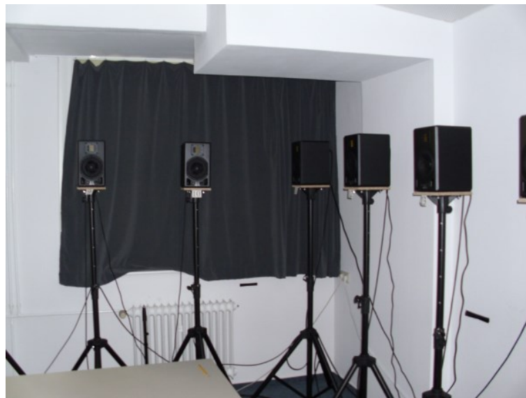
Figure A.2.: Photo from the loudspeaker surrounding system in the wave field synthesis room in the Institute of Musicology at the University of Hamburg.
