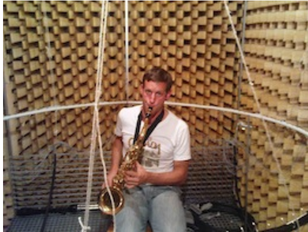
Figure 5.1.: Photo of the measurement setup recording the radiation characteristic of a tenor saxophone. The microphones stick out of the circular rim as can be seen in the lower-right corner.
