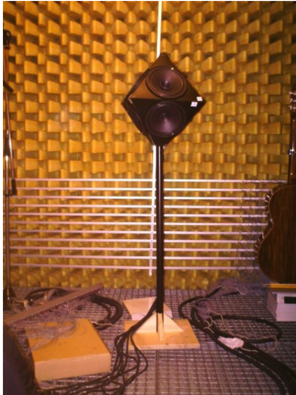
Figure A.1.: Photo of the octupole speaker system in the free field room.
