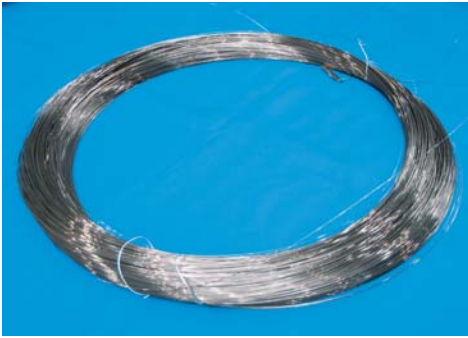
Fig. 5: Final single piece multifilament wire in batch size exceeding 1000 m (Bruker EAS).
