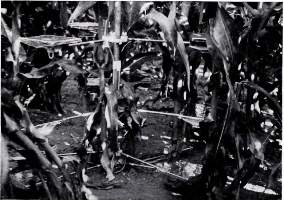
Fig. 2. Sensors under radiation protection screens, relatively close to the soil surface. The photograph was made at the end of August, between 17h00 and 18h00, with a solar altitude of about 15° (Photograph J. van den Brink).
