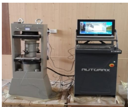
Figure 2. Static-elastic modulus test for geopolymer concrete tested at 28 days
