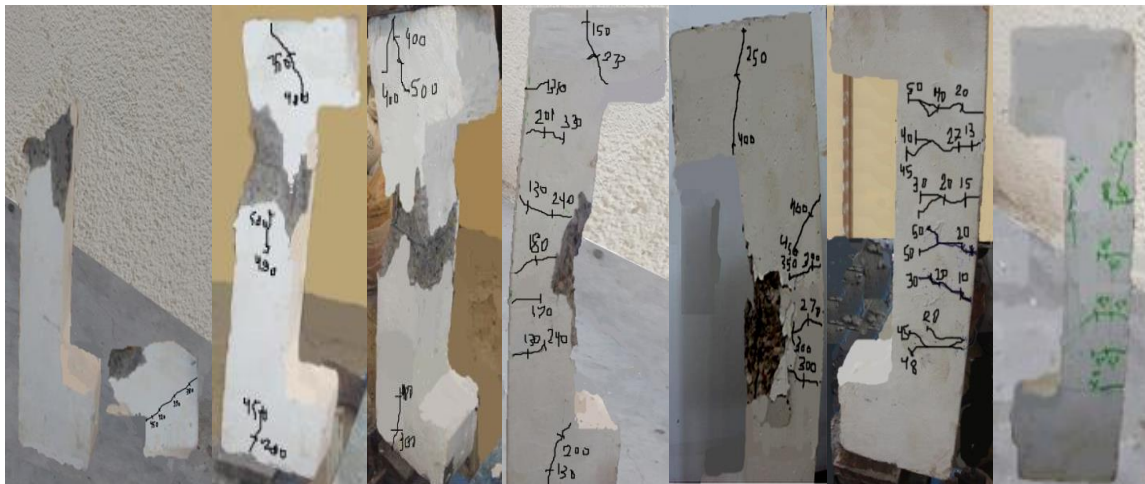
Figure 9. Cracks pattern of failure
