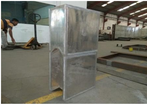
Fig 9a. Shielding construction of paraffin block
