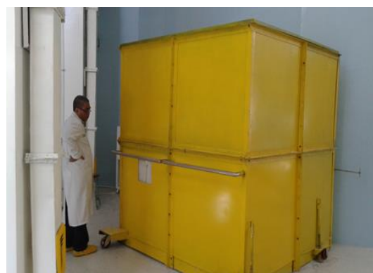
Fig 8. Final Revitalization of cubical paraffin shielding (2 x 2 x 2)m 3
