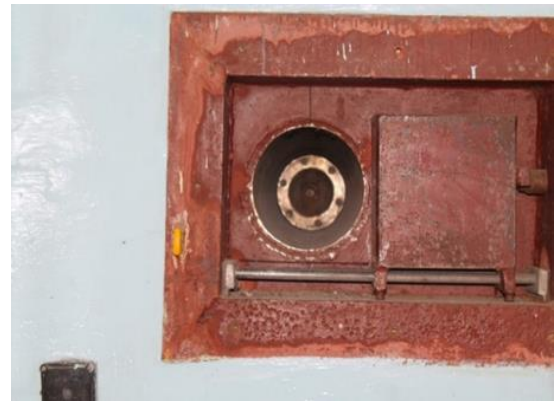
Fig 5. The actual radial piercing beamport neutron source of Kartini Reactor.
