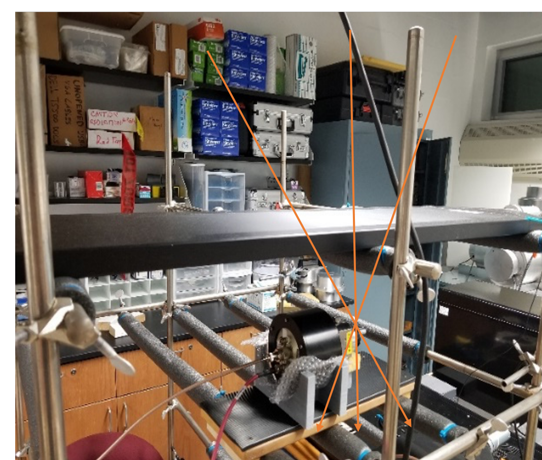
Figure 2: Top detector is an EJ-200 plastic scintillator. The bottom detector is the Xylene detector.
