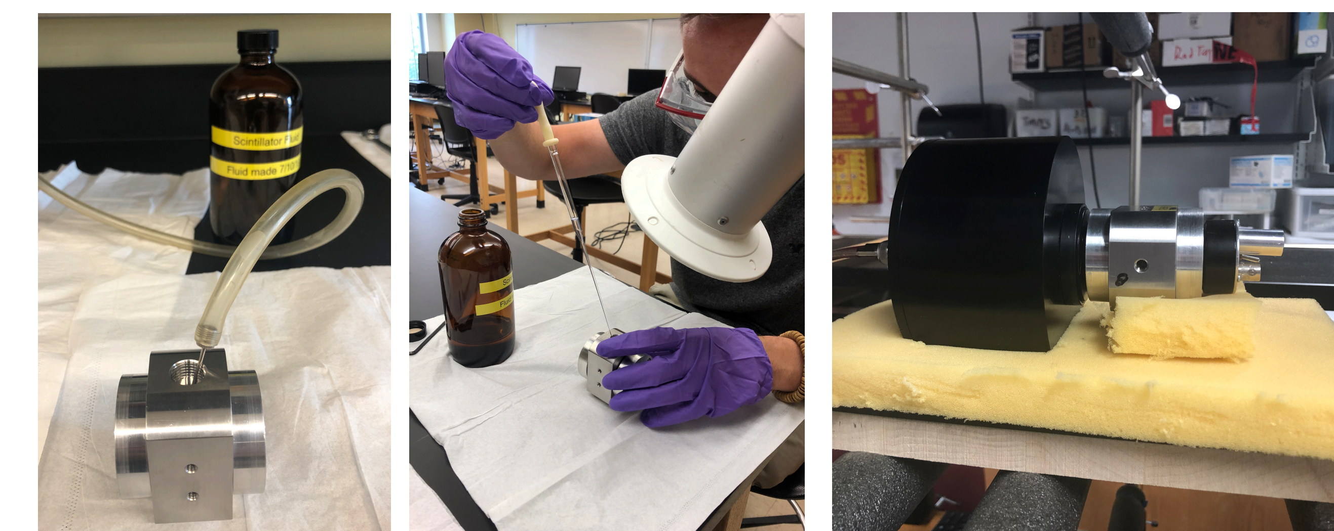
Figure 7: Bubbling oxygen in xylene detector (left). Matthew Signor filling the xylene detector with the scintillator fluid (middle). Small Xylene vessel attached to the Photech PMT 240
