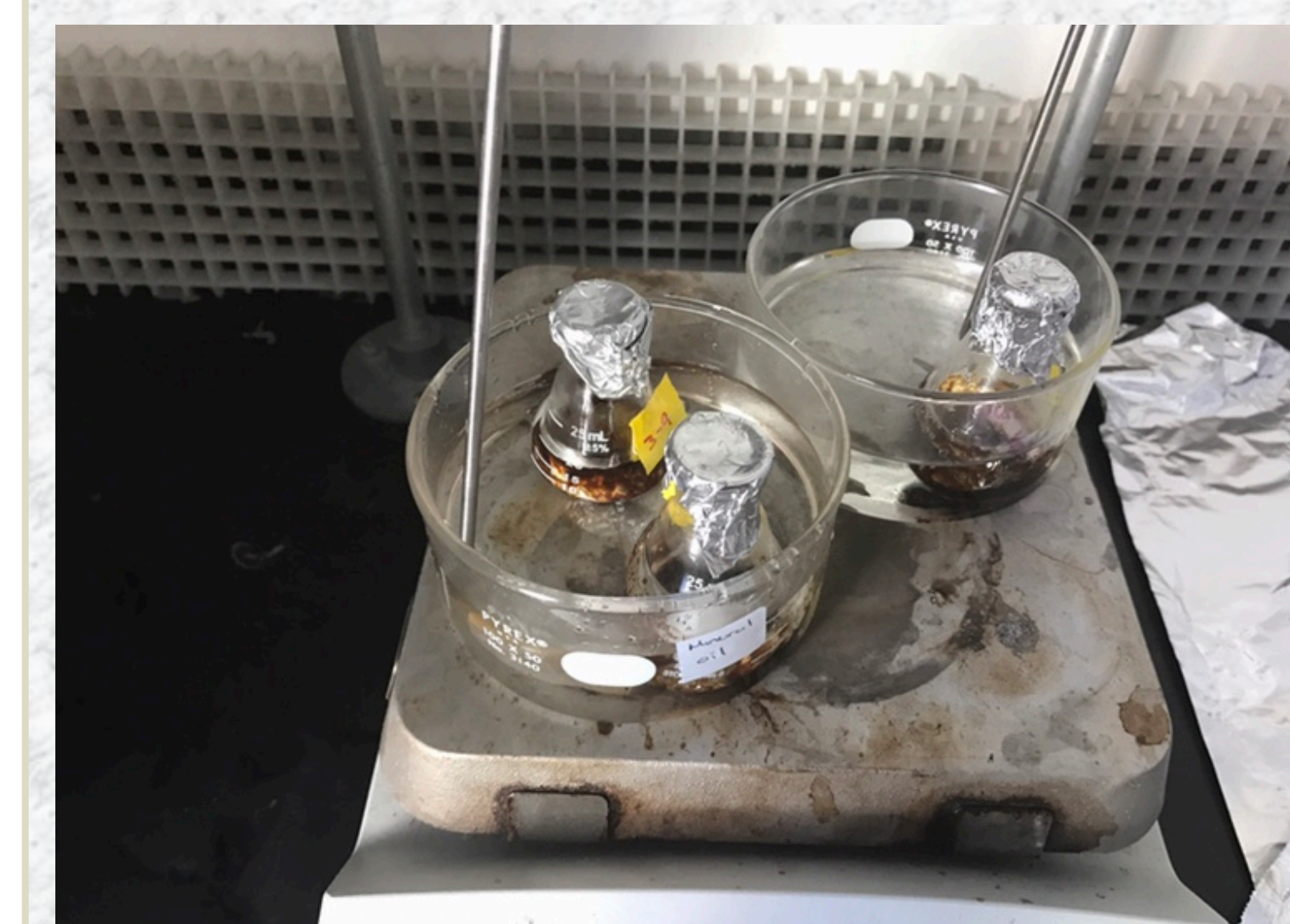
Figure 3. Acid Hydrolysis of Ground Alfalfa Hay and Ionic Liquid
