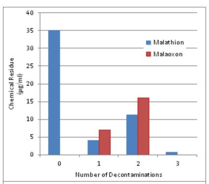
Mean malathion and malaoxon residuals ( $\mu g/ml$ ) on steel plates after 0, 1, 2, or 3 applications of 5% sodium hypochlorite (bleach) solution applied with an air brush.
