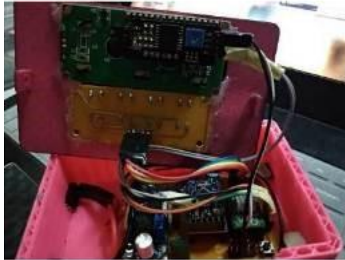
Gambar 6. Connection of LCD display and push buttons.
