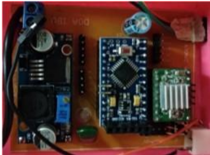
Gambar 5. Voltage step down, microcontroller and motor driver.
