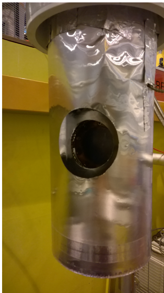
Figure 10.3: Modified in-situ ice growth set up with two aluminium heat shields with "beam in" and "beam out" holes in front of and behind the vanadium plate. Photo credit: Tristan Youngs (ISIS)
