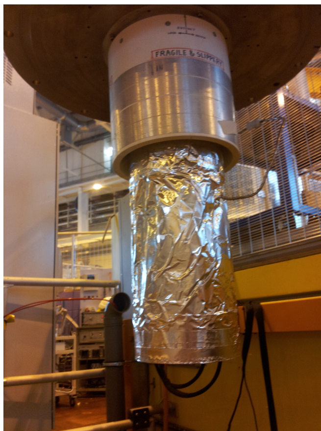
Figure 6.9: Photograph of the aluminium 10 K that surrounds the set up to lower the base temperature of the vanadium plate.
