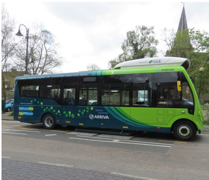
Figure 7.5: A Milton Keynes eBus in service in April 2014 charging on an inductive plate in Wolverton
