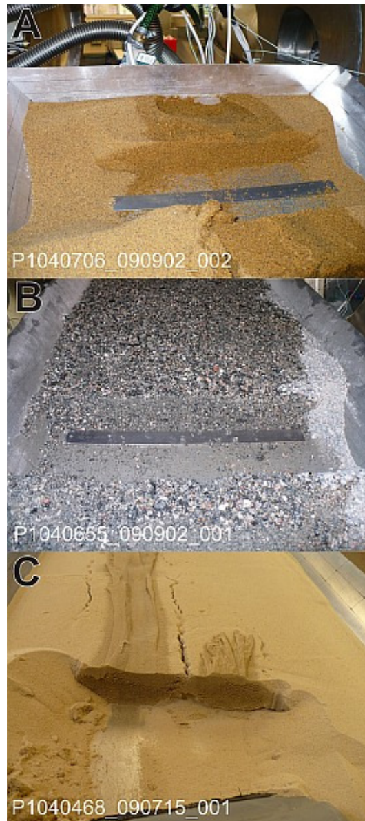
Figure 8-7. Wetted areas for the three sediment types under ambient temperature/ambient pressure with the photo ID followed by the experiment ID in the bottom left of each photo. A: medium sand showing 1-2cm infiltration halo on the surface and wider halo sub-surface, making an oval shape in cross section. Water has percolated to the end of the tray. B: rock crush showing wide wetted area from flow and vertical boundary between wet and dry. C: fine sand showing narrow percolation halo at the surface and wider percolation halo underneath, giving an oval cross section. Cracks in the surface of the sand indicate the lateral extent of the wetted area beneath the flow. Lobe to the left is ~15cm wide at widest point.
