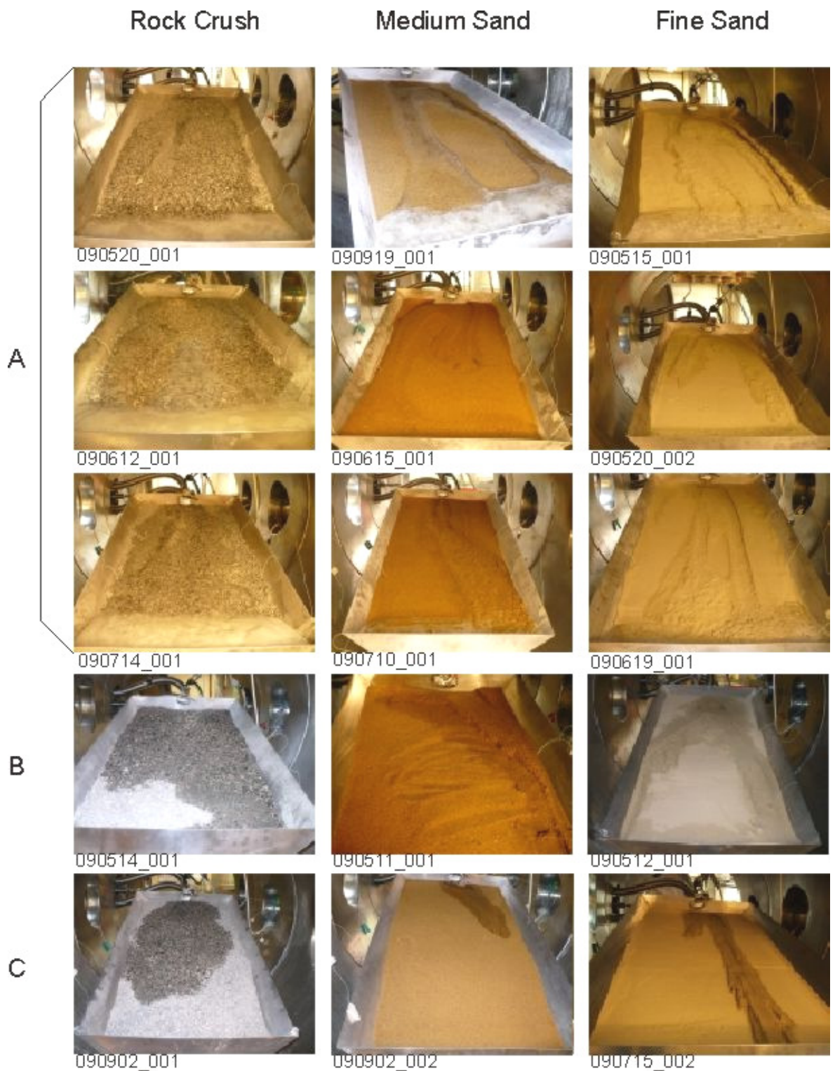
Figure 8-5. Matrix of photographs for each experiment when complete, each column vertically is a different sediment type and each row represents different ambient experiment conditions, with A being low temperature/low pressure, B ambient temperature/low pressure and C ambient temperature/ambient pressure.
