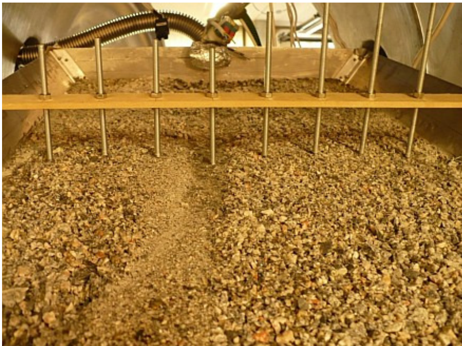
Figure 8-2. Photograph of profiler used to measure cross sections for volume calculations. The tray is 54 cm across at the top.
