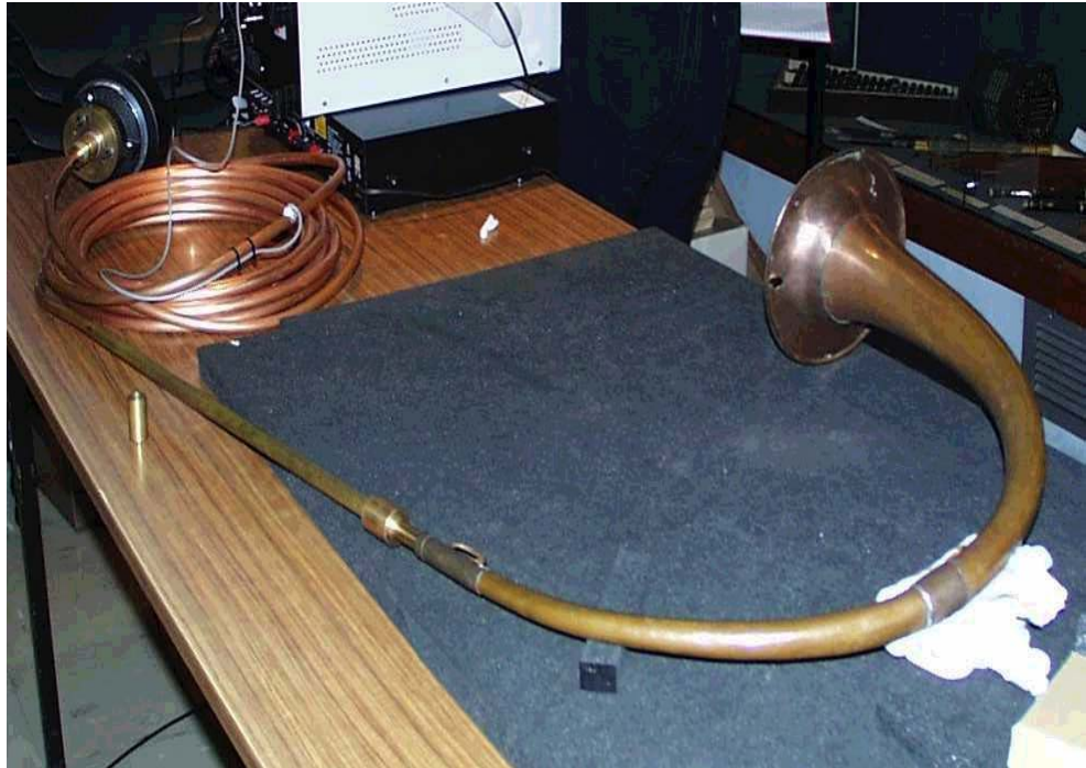
Figure 6.9: 18 th century Bugle Horn coupled to pulse reflectometer
