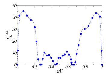
FIG. 10. (Color online) Axial component of cross-flow energy. Associated with the order-3 ring-bursting pattern for Re = 545, time averaged axisymmetric energy component  $\overline{E}_0^{cf,z}$ . Note that all higher azimuthal wave numbers are on the order of  $10^{-4}$ .
