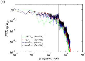
FIG. 6. (Color online) Power spectral density (PSD). PSD curves calculated from the radial flow component  $u_{d/2} = u(d/2,0,\Gamma/2,t)$  for (a) WVF<sub>39</sub> for Re = 500 and (b) ring burst of order-3 for Re = 545. (c) PSD curves scaled by the respective Reynolds number for different flow patterns. As the number of ring bursts is increased, the local peaks in the PSD curves become more pronounced. The vertical line highlights the resemblance of the spectra.
