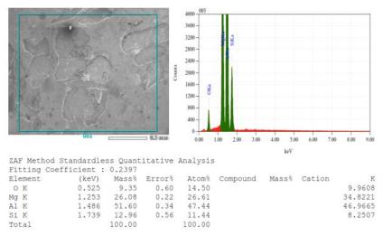
FIGURE 7. SEM+EDS Data of Al-Mg-Si Composite after Quenching Process
