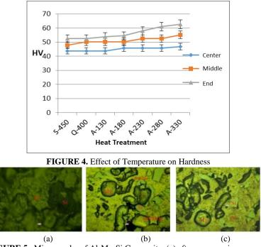
FIGURE 5. Micrography of Al-Mg-Si Composite; (a).after compression process; (b). after quenching process; and (c). after aging process.
