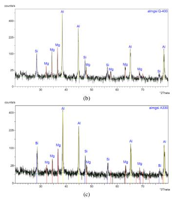
FIGURE 6. XRD Pattern of Al-Mg-Si Composite: (a).after compression process; (b). after quenching process; and (c). after aging process.
