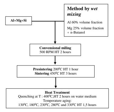
FIGURE 3. Flowchart of Sample Preparation
