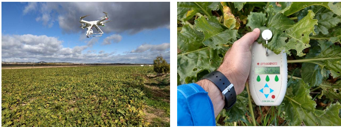
Figure 3. (Left) Unmanned aerial vehicle used for field data collection; (right) measurement with CCM-200 chlorophyll meter.
