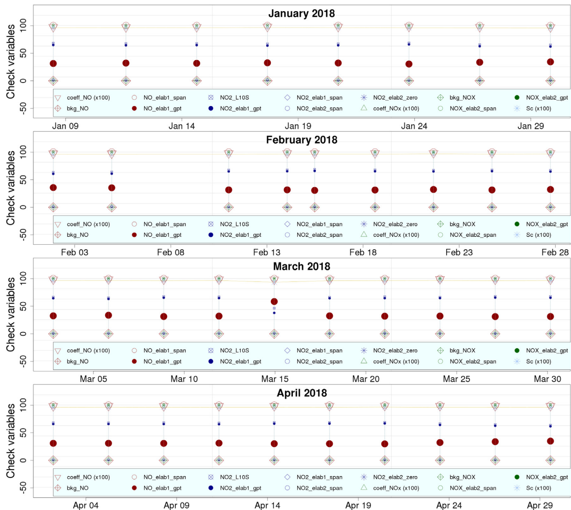
Fig. 4. Time series of calibration factors (bkg_NO, coeff_NO, bkg_NOx, coeff_NOx, Sc) and NO-NO 2 -NO x values during the different steps of calibration events, from January to April 2018 at CMN (NO_elab1_span, NO_elab1_gpt, NO 2 _elab1_span, NO 2 _elab1_gpt, NO 2 _elab2_span, NO 2 _elab2_zero, NO x _elab2_span, NO x _elab2_gpt).
