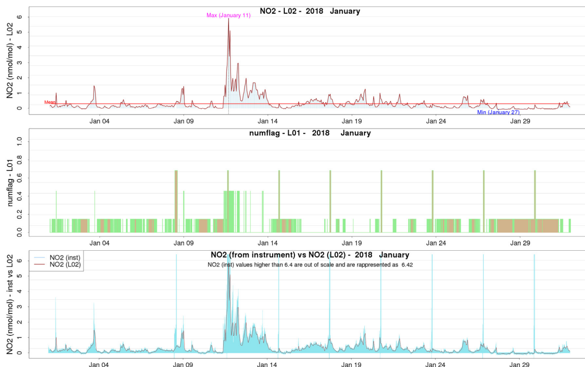
Fig. 5. Upper: NO 2 (Level-2) at CMN in January 2018. The average value (red flat line) is also reported, together with the minimum (Min) and the maximum (Max) values for each month. Middle: numflag for NO 2 1-min data (Level-1). Bottom: comparison between Level-2 data (red line) and raw 1-min readings from the instrument (blue area).
