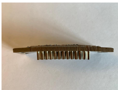
(a) Cross section of the IGBT module
