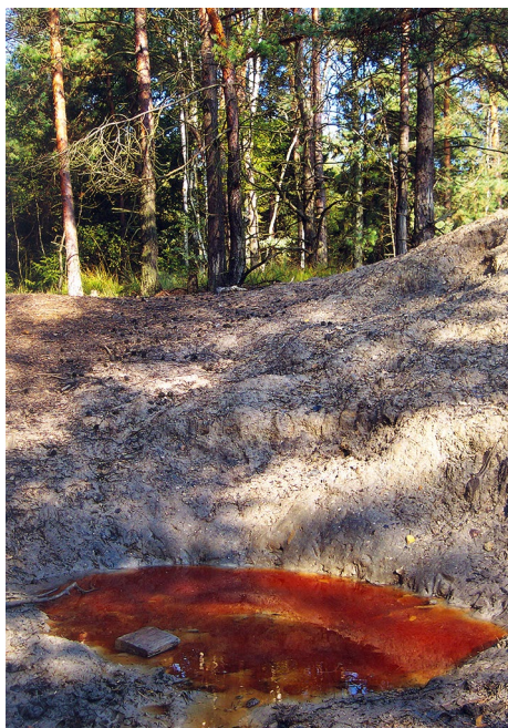
Fig. 5 Acidic leachate (pH < 2, the average: EC—5.9 mS/cm, SO 4 2- —4800 mg/dm)
