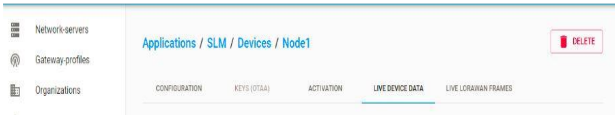
Figure 4. 1: LoRa App server showing an application-SLM and a device-Node1 created
