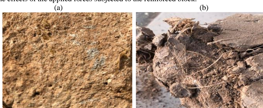
Figure 6: (a) Sample block with bamboo fibres and (b) the failure mode of the reinforced block under compressive tests.
