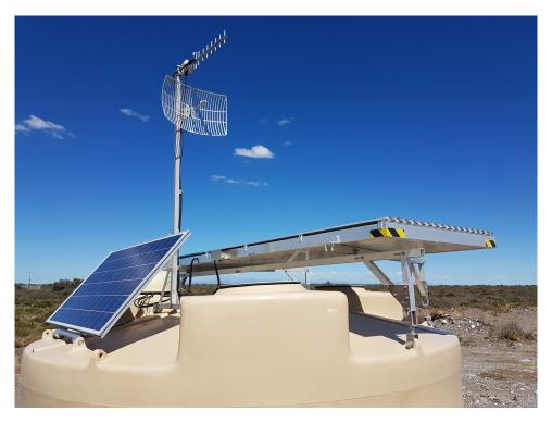
Figure 2.7: A sample photograph of an SSD deployed in the standard array above a WCD.
