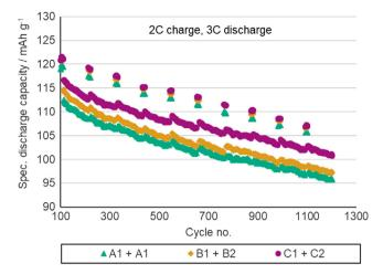
**Figure 11.** Long-term stability of multilayer electrodes. The cells were charged with 2C and discharged with 3C from cycle 100 to cycle 1200. Every 100 cycles, there are some 1C/1C steps for reference. The sample C1 + C2 with the highest binder gradient during coating shows the highest discharge capacity.
