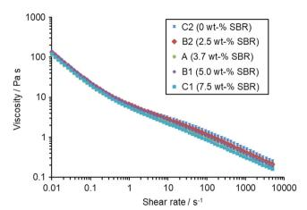
**Figure 2.** Average viscosity of the different anode slurries as a function of the applied shear rate. All slurries show a very strong shear thinning behavior. With addition of SBR binder, the solid content is reduced, and thus the viscosity is reduced.
