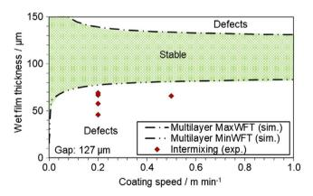
**Figure 8.** Coating window with observed process points of intermixing of both layers. The simulated process limits for the minimum wet film thickness MinWFT and the maximum wet film thickness MaxWFT are shown.
