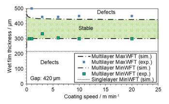
Figure 5. Coating window for the simultaneous two-layer coating of anode slurry with a coating gap of  $420 \,\mu m$  (high-energy cells).
