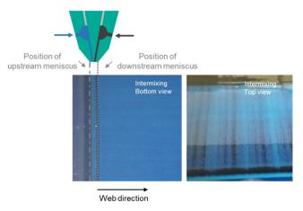
**Figure 7.** Examples of top and bottom views with intermixing of both layers. Gap  $h_{\rm G} = 127 \,\mu{\rm m}$ . Web speed  $u_{\rm web} = 0.2 \,{\rm m \,min^{-1}}$ . Wet film thickness  $h_{\rm wft} = 69 \,\mu{\rm m}$  (50% top layer and 50% bottom layer).
