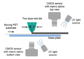
**Figure 12.** Coating setup for the investigation of coating stability and for characterization of the coating window with a two-layer slot die and two CMOS sensors and UV light sources for film inspection.
