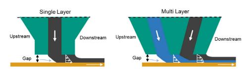
Figure 6. Schematic flow profile at the limit to the minimum wet film thickness for single layers (left) and multilayers (right).
