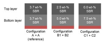
**Figure 1.** Schematic cross section of the multilayer stacks. Numbers indicate the different contents of SBR binder in wt%. Configuration A + A is the reference electrode with the same amount of SBR binder in top and bottom layers. Configuration B1 + B2 is two-thirds of the SBR binder in the bottom and only one-third in the top layer. In C1 + C2, the SBR binder is only in the bottom layer during coating.
