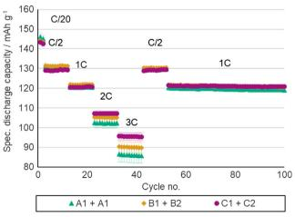
Figure 10. Specific discharge capacity of full cells for layer configuration A + A, B1 + B2, and C1 + C2 for normal capacity of 2.05  $\pm$  0.08 mAh cm<sup>-2</sup>.
