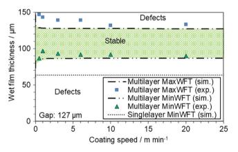
**Figure 4.** Coating window for the simultaneous two-layer coating of anode slurry with a coating gap of 127  $\mu$ m (state-of-the-art thickness). The stability behavior was also simulated according to Schmitt et al.<sup>[16]</sup>
