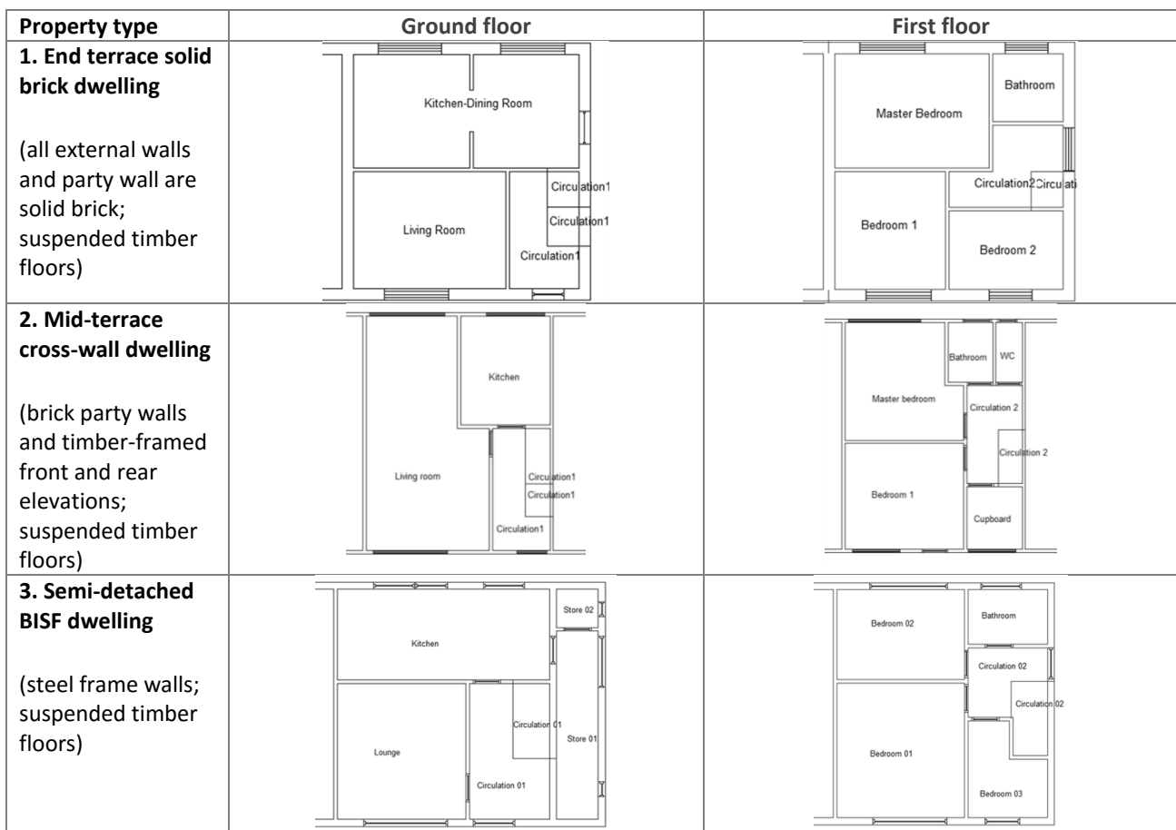
Figure 2: The typical social houses selected for the study (note that north is towards the top of the page in all plans)
