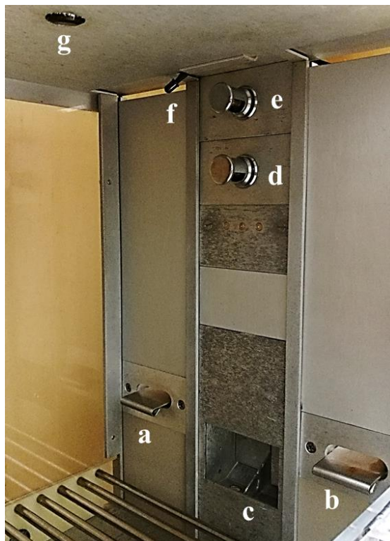
Figure 7. Operant chamber used to carry out behavioural experiments. On the frontal panel is possible to note the right lever (a), the left lever (b), the food dispenser placed in between the two levers (c), the red house light (d), the white house light (e) right above the white one, the infrared emitting diode (f) and the video camera (g). All the Skinner boxes were placed inside a sound-isolated cubicle equipped with a fan providing ventilation and a background white noise.
