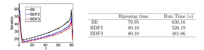
FIGURE 6. Ripening time of 2D CH equation with small fixed time ( $\Delta t = 0.01$ )
