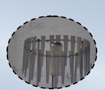
Heated (49 W) tipping bucket with single-Alter shield
