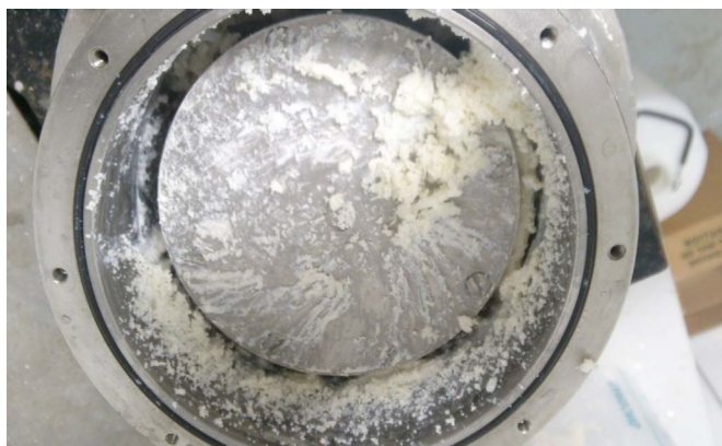
Fig. 5. Severe fouling in SDR at low ratio of water/TTIP = 4 [22].
