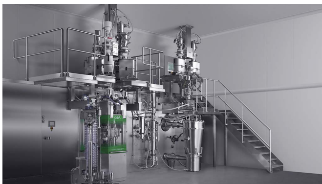
Fig. 25. A ConsiGma unit in Pfizer Lab at Groton, United States for the investigation into on-demand tablet production [105].
