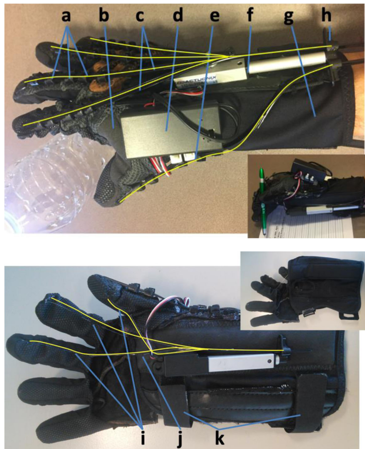
Fig. 1 The HERO Grip Glove assists finger and thumb extension and flexion to enable users to grasp large and small objects. The HERO Grip Glove consists of (a) cable tie guides, (b) an open-palm glove, (c) cable tie tendons for extension, (d) a 9V battery case with the battery inside and the microcontroller with an inertial measurement unit mounted between the case and the glove, (e) buttons to control the manual mode and select between the manual and automatic modes used in [14], (f) a linear actuator, (g) a foldable wrist brace, (h) cable tie pawls for pre-tensioning, (i) fishing wire tendons for flexion, (j) tendon anchor points on the wrist brace and (k) Velcro straps to secure the glove. The glove folds open to ease donning. The dorsal and palmar tendons' routing paths are highlighted in yellow
