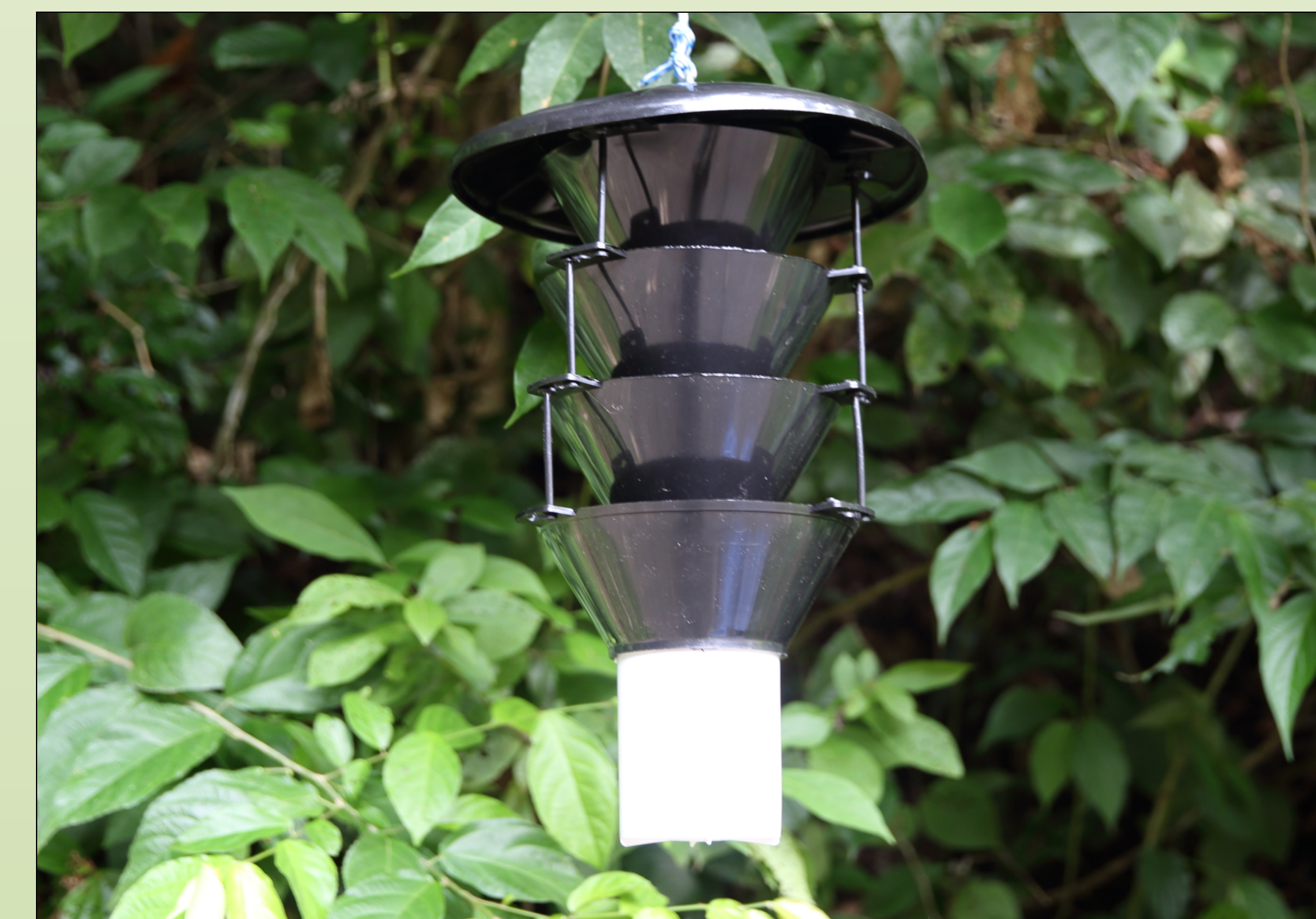
Figure 5. Lindgren Funnel (Flight intercept trap)
