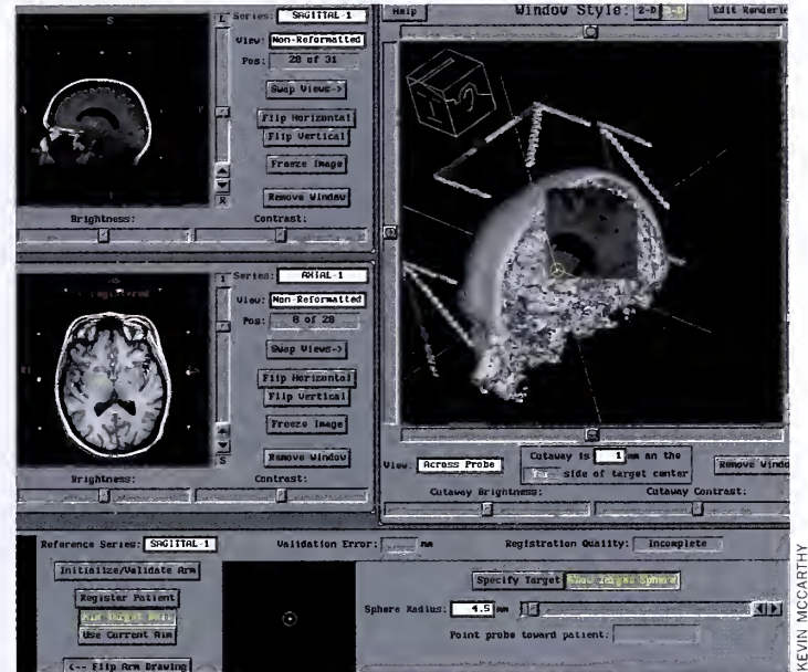
Magnetic resonance images of the brain, shown above, along with electrophysiology recordings, are used to identify the approximate locations of seizure-generating brain tissue. Using a stereotactic frame, the tissue to be studied is targeted (intersection of yellow lines) and a trajectory plotted. An electrode may then be inserted precisely.
