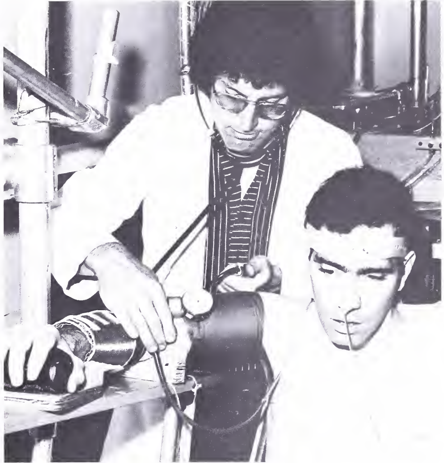
Changes in skin blood flow and peripheral pooling of blood are important consequences of exposure to heat and exercise. Dr. Ethan R. Nadel, left, is adjusting capacitance plethysmographs which make it possible to measure forearm skin blood flow in an exercising subject.
