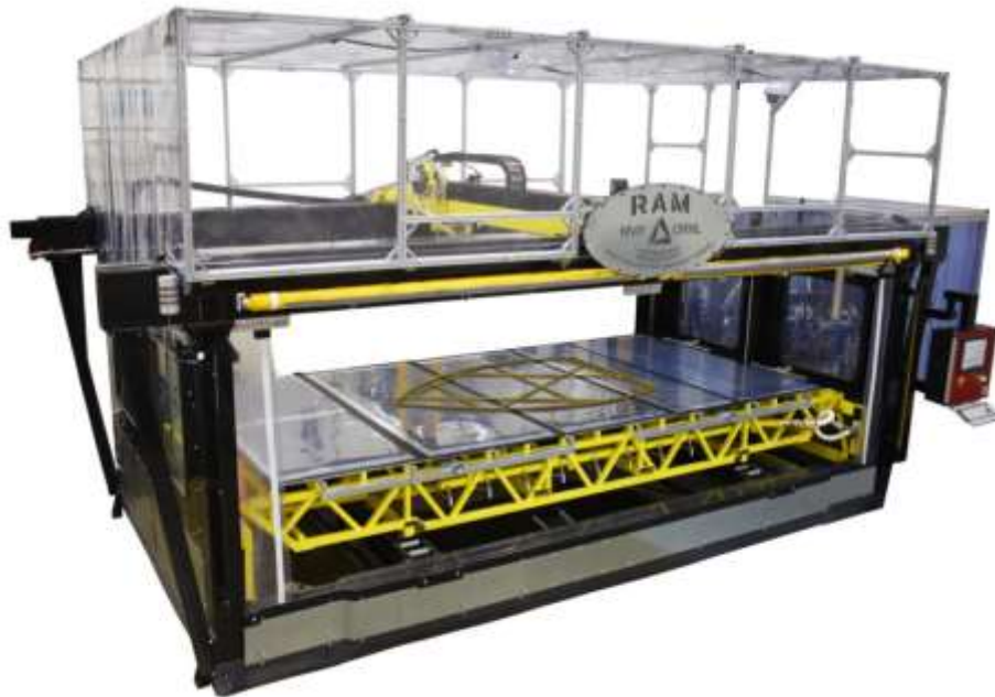
Figure 1 – The Reactive Additive Manufacturing (RAM) printer produced by Magnum Venus Products in collaboration with Oak Ridge National Laboratory.
