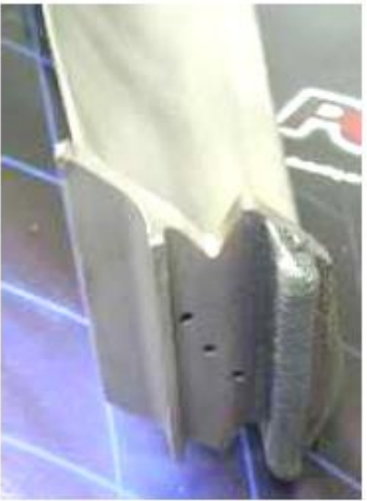
KNIFE EDGE BUILDUP Base Material : Inc 738 Filler Material: Inc 625/617 Deposition speed: 400 mm/min
