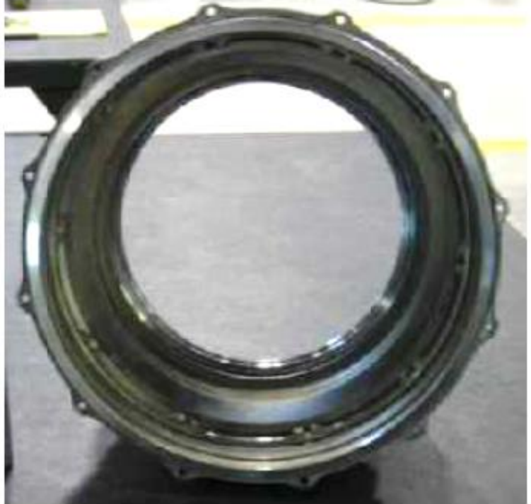
Rebuild Flanges Filler Material: IN625
