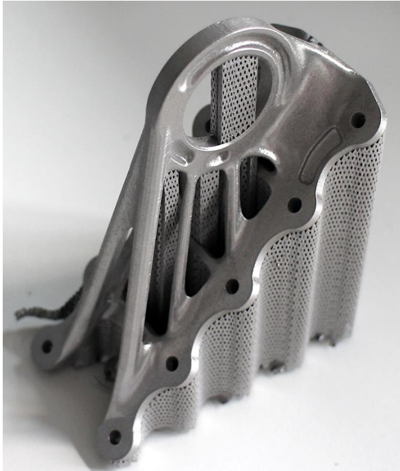
Custom Porous Metal, Designed Via Laser Sinter
