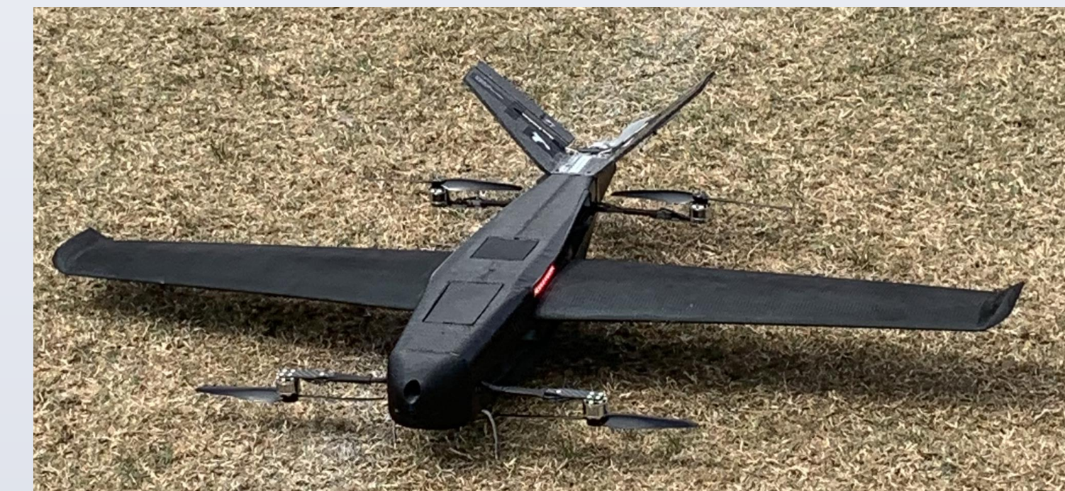
Figure 5. Krossblade Skyproowler 2 with VTOL rotors extended.
