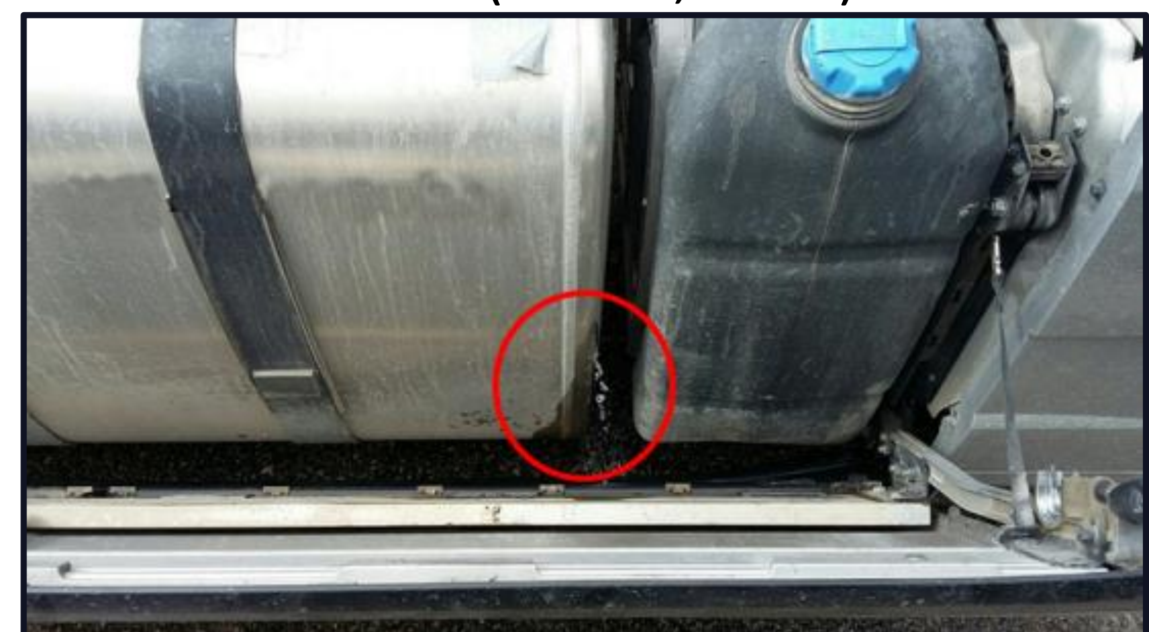
Figure 3. Internal cracks in the Volvo bus fuel tank
