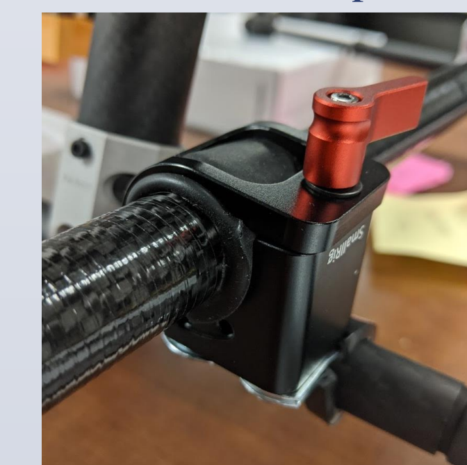
Figure 6. Close up of quick release clamp used to attach anemometer boom to the landing gear. Also imaged: layer of vibration isolation material.
