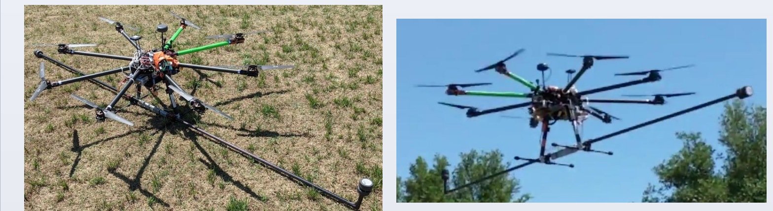
Figure 5. Fully instrumented unmanned aircraft. microcontroller, power supply, data storage and telemetry are centrally located with all meteorological instruments mounted on booms: (a) on the ground; (b) in the air.
