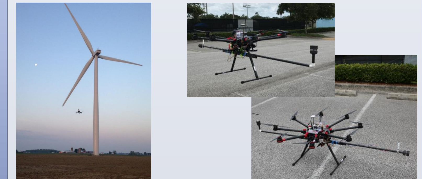
Figure 5: (Left) Measurements were made around a single upstream GE 1.7 MW wind turbine with an 80 m hub height and 100 m rotor diameter. (Right) Fully instrumented unmanned aircraft, microcontroller, power supply, data storage and telemetry are centrally located with all meteorological instruments mounted on booms: (a) on the ground; (b) in the air.
