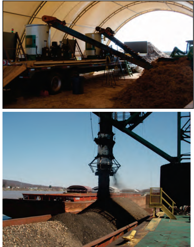
Figure 1. Mobile briquetting units (above) and pelleted switchgrass being loaded on a barge with coal (below).
