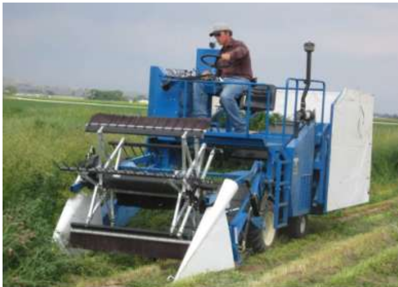
Fig. 1 Powell Research and Extension Center: Forage harvesting using a Swift forage harvester.
