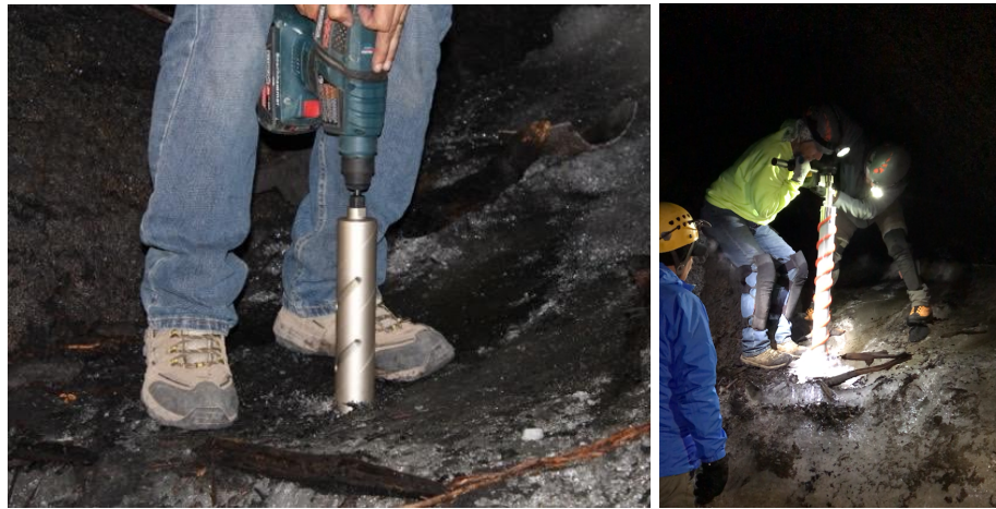
Figure 10: Left: Coring the ice deposit from the floor of Cave 91. Right: Image of the recovered ice core.
