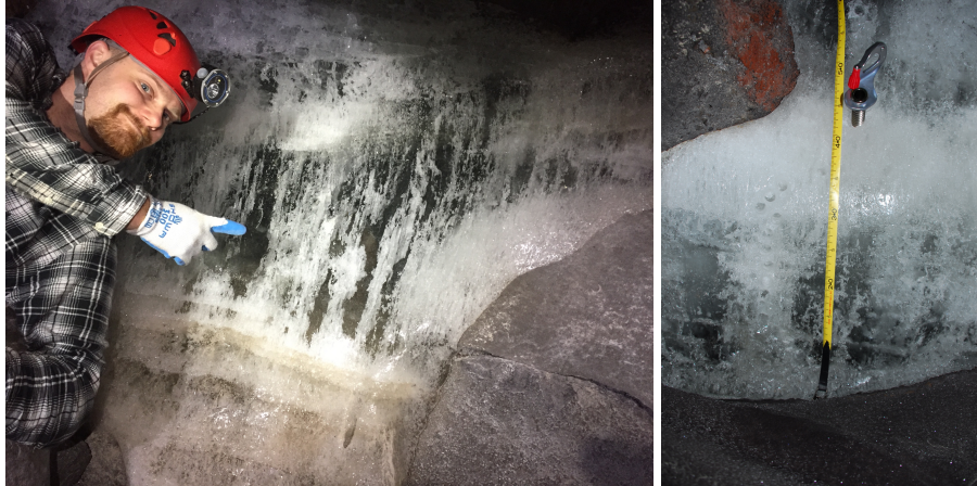
Figure 12: Left: The ice wall in Cave 455. Right: Recovering short, horizontal ice cores at 2-cm intervals using a Petzl ice screw on the ice wall of Cave 455.
