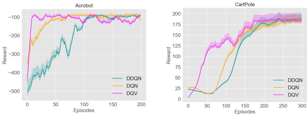
Figure 2: The results that have been obtained when using DQV in combination with an MLP on two classic RL problems (Acrobot and Cartpole). DQV learns significantly faster when compared with DQN and DDQN.
