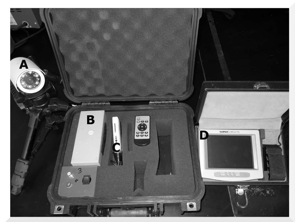
Fig 1. Digital camera system. The surveillance camera (A) is connected to a padded Pelican™ case, which contains a battery supply (B) and a mini-DVR (C). The monitor (D) can be connected to the system during setup in the field to ensure the seed station is properly focused within the camera's field of view.
