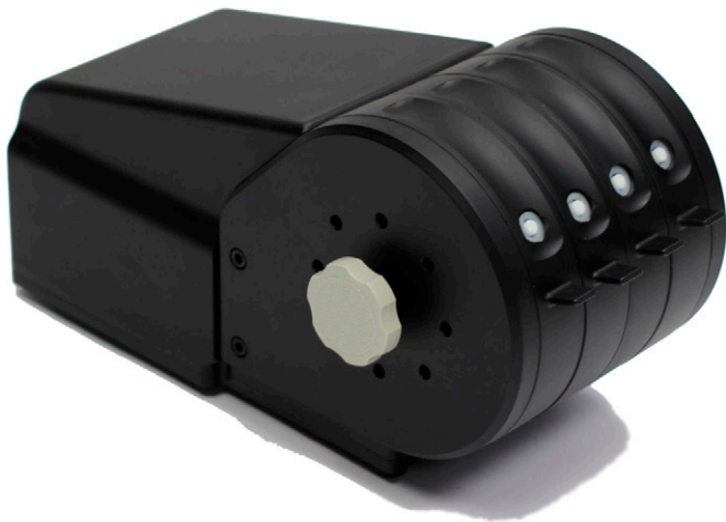
FIGURE 1. Four-site vibrotactile stimulator. Each of the four probe tips was positioned by rotating the four independently positioned drums to maximize contact between finger pads and the simulator tips.
