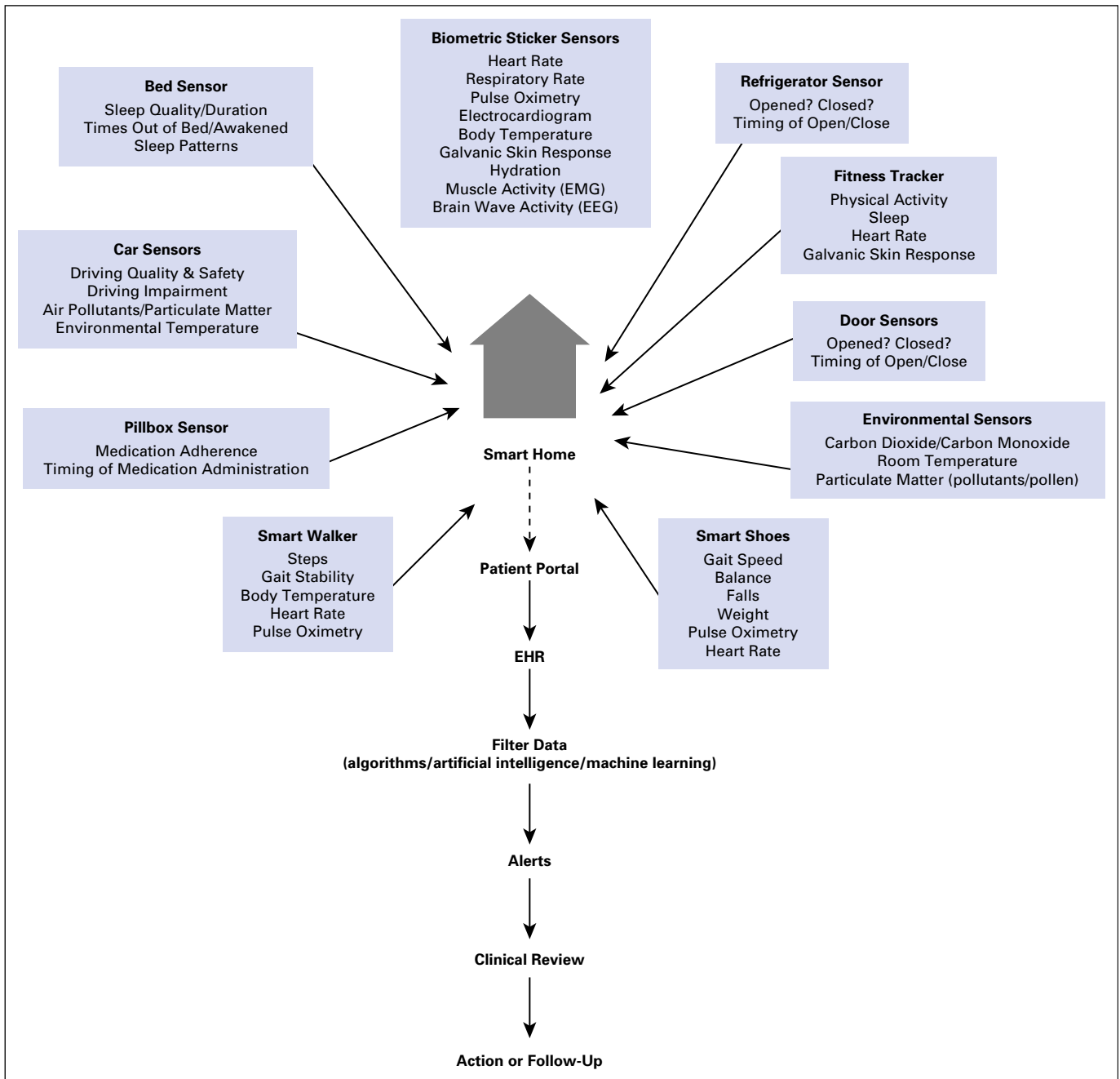
FIG 1. Conceptual model of an “Internet of Things” ecosystem for health. EEG, electroencephalogram; EHR, electronic health record; EMG, electromyogram.
