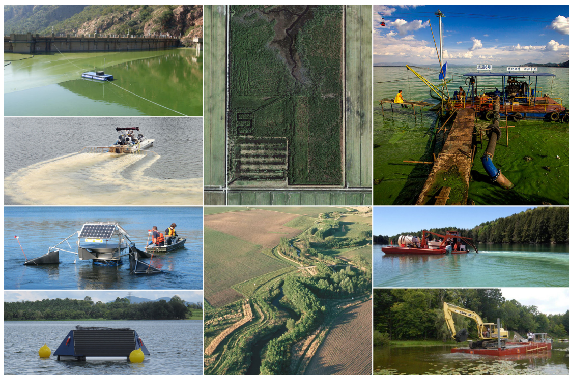
Fig. 3. (Clockwise from top left) Floating booms at Hartbeespoort Dam, located in the North West Province of South Africa, are used to concentrate cyanobacteria so they can be pumped out and composted (photo credit: Dept. of Water and Sanitation, Republic of South Africa); a constructed wetland at Open Grounds Farm, near Beaufort, NC, designed to reduce the amount of nutrients and sediments entering the headwaters of the South River, a tributary of the Neuse River (credit: Google Earth); a pumping barge is used to remove harmful cyanobacteria from Dianchi Lake, China (photo credit: J. Carl Ganter/Circle of Blue); aluminum sulfate and sodium aluminate are pumped into Ticklenaked Pond in Ryegate, VT, to combat phosphorus loading and harmful cyanobacterial blooms (photo credit: Vermont Dept. of Env. Conservation, Watershed Management Div.); a dredging operation in Lake Roaming Rock, Ohio, to remove nutrient-rich sediments (photo credit: RomeRock Association); a riparian buffer along Bear Creek in Story County, Iowa, designed to filter runoff of nutrients and sediments from adjacent farmland (photo credit: USDA); a LG Sonic, MPC-Buoy uses ultrasound waves to control algae (photo credit: LG Sonic); a SolarBee solar water circulator, used to reduce surface algae blooms in Santuit Pond in Mashpee, Massachusetts (photo credit: Friends of Santuit Pond); Phoslock is applied to Laguna Niguel Lake, CA, to bind and remove phosphorus from the water column (photo credit: Aquatechnex).
